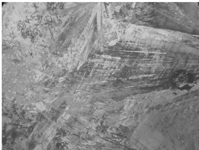
FIGURE 2 Polarized micrograph for compound 1–7 at 255°C.
